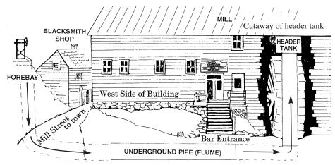
Water from the Vantine Brook flows through the upper raceway into the forebay. Water is discharged from the forebay, under Mill Street, through a three-foot pipe (flume) on the way to the header tank at the top of the wheel. The water flow is fed by gravity; there is no pump.
